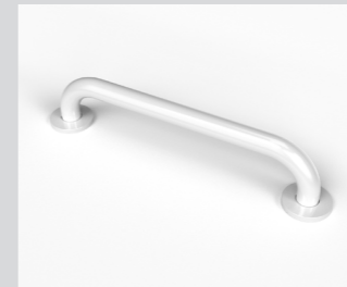
455mm straight grab rail Powder coated stainless steel Doc M and HBN compliant. W455 x Ø35mm Code: White GRAB201 Blue GRAB204 Light Grey GRAB207 Dark Grey GRAB210
